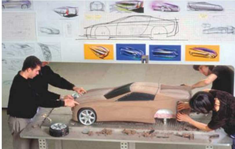
Figure 1: Designers working on a clay model of a car
